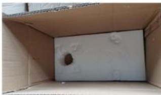
1.Put polyurethane foam inside
