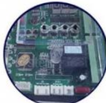
Brush-less DC Control board
