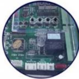
Brush-less DC Control board
