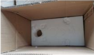
1.Put polyurethane foam inside
