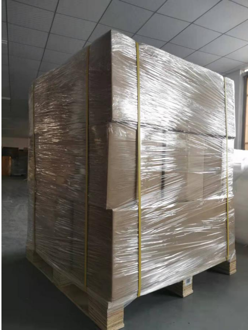
2.Cover with plastic and put the motor into the carton
